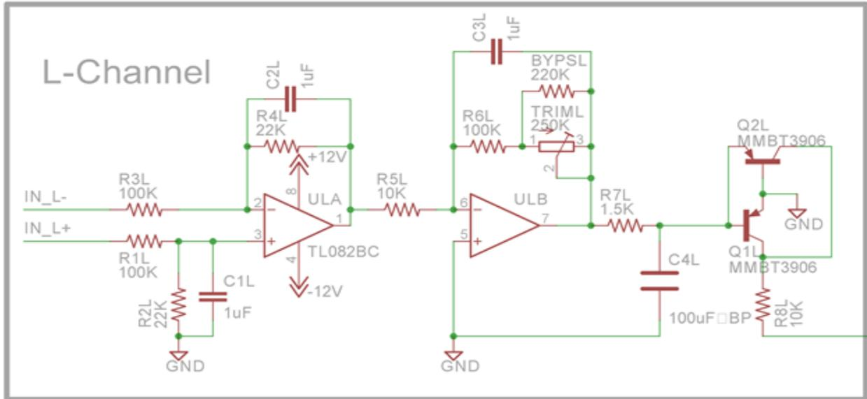
The left channel is included in the figure above, with the right channel being an identical copy. The only difference is the use of a suffix *R* instead of *L* for part names.
