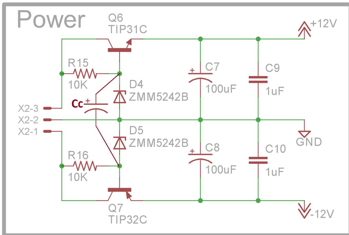
The capacitor Cc will be used as a charge reservoir in the event of switching, and will stop this multiple triggering effect from occurring.
