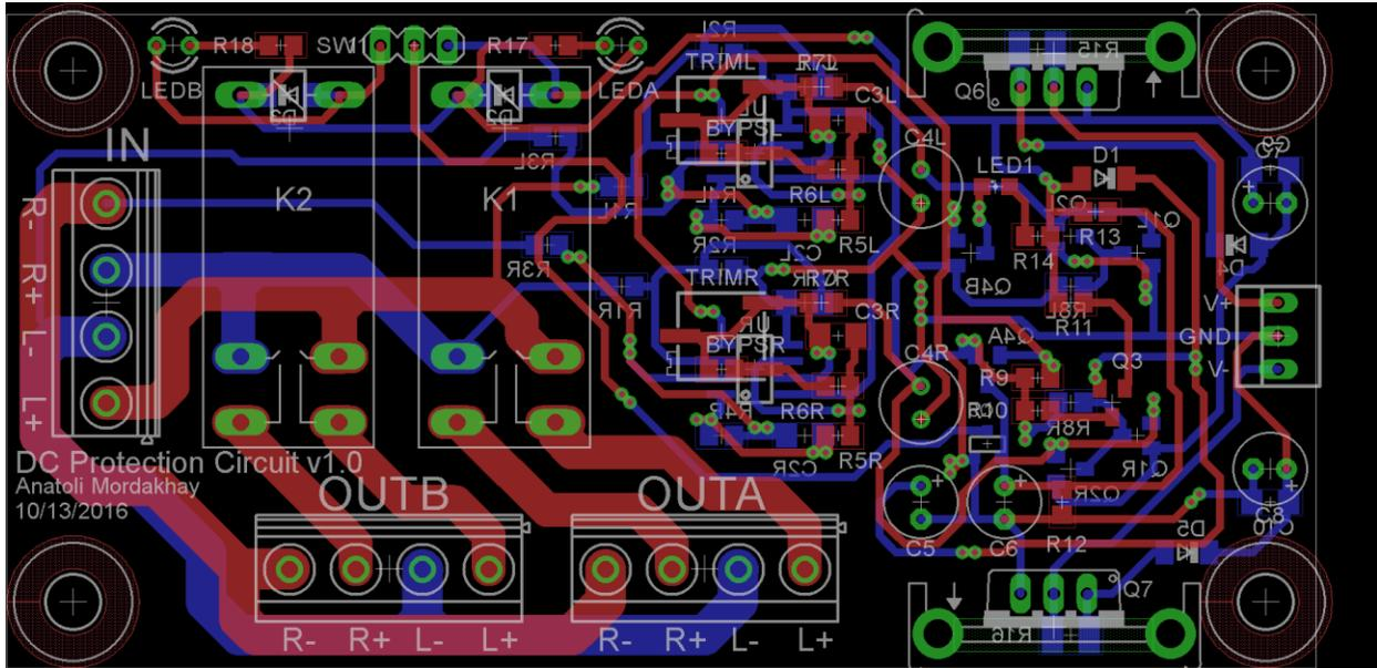
It is a 2-layer board. The signal lines are wide to support high current, and all of the filtering/switching elements are placed far from the signal lines. This is done to minimize any interference to the signal lines.
