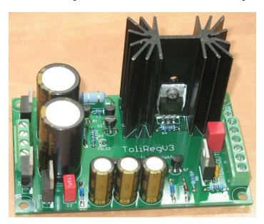
The board was set to 32VDC, with a current limit of  $\sim$ 1.5A (0.47ohm Rsense), with an input capacitance of 4400uF (2x2200uF).
